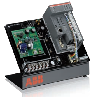
PLC-trainer ABB AC500 with plug-on motor module
